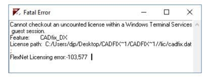
The user is accessing a CADfix client machine via Terminal Services to run CADfix. The CADfix license is node locked to only allows CADfix use on the client machine, not the display computer where the user is located.
