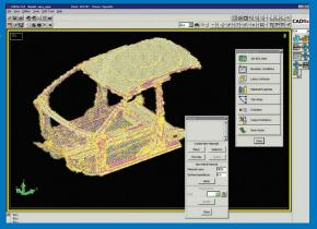
The geometry and meshing requirements of the EMC division are quite different from those of other disciplines at MIRA. The crash testing division, for example, needs to model the structure and major metal parts, but if they are working on a frontal crash model they might chop off the back of the car and replace it with a generic mass.
