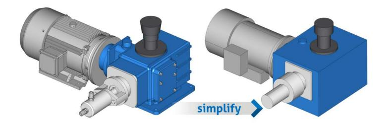
CADfix PPS generates lightweight simplified versions of CAD models to meet the demands of downstream applications, where the full detail of the mechanical CAD model is not required, but the overall aesthetic is needed for visualization, positioning, and packaging. CADfix PPS achieves significant reductions in model size and complexity whilst retaining the key features of the source CAD model.
